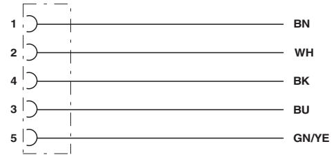
Contact assignment of the M12 sockets
